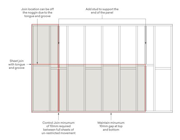
W Use of butt joints between panels ends will not be recognized under warranty.
