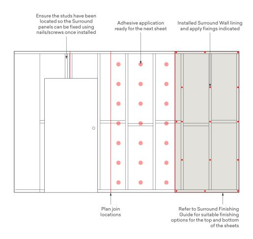
Apply generous amounts of construction adhesive on each stud/ noggin behind each Surround by Laminex panel. It is recommended to follow the adhesive manufacturer's instructions for the amount to be used.
