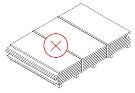
All straps and restraint devices must remain grit and burr free and suitably tensioned to prevent movement of the product during transport. Covered loads are recommended to prevent damage during transport to site.
