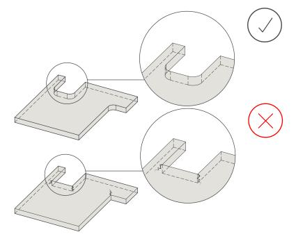
Cut-outs can be made with a router or by pre-drilling a hole with an appropriate diameter drill bit to meet internal radius requirements and then cut between drill holes.
