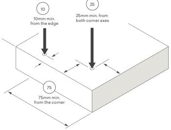
When applying fixings with power tools (nail gun, screw gun) only use enough pressure to drive the head of the nail or screw marginally below the surface of the panel. Splitting of the panel can occur if the pressure is too high or if the fixing is driven in too far and tooling marks will show on the finished surface.
