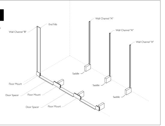
Locate all divisional panels into the rear channels "A" resting onto the saddles.
