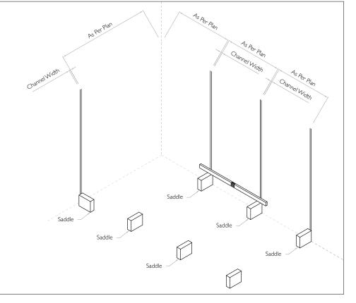
Fix channel "A" to back wall by placing on top of the leveled saddles.
