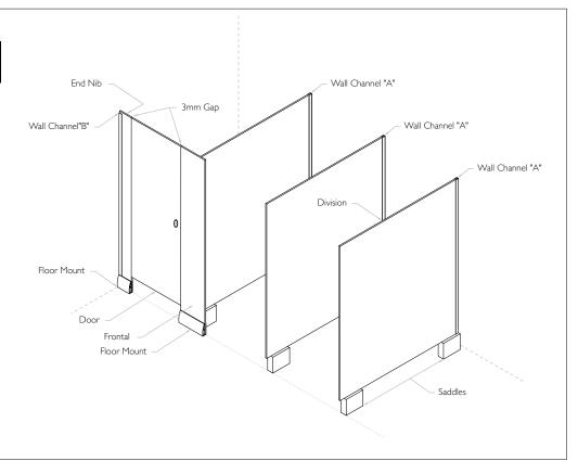
When all cubicles have been assembled, place a string line across the fronts at the top of the cubicles.
