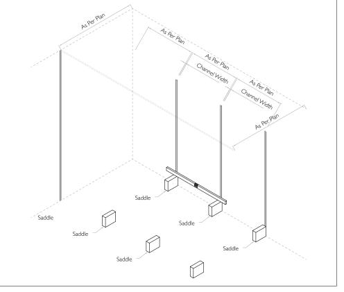
Fix channel "A" to back wall by placing on top of the levelled saddles.
