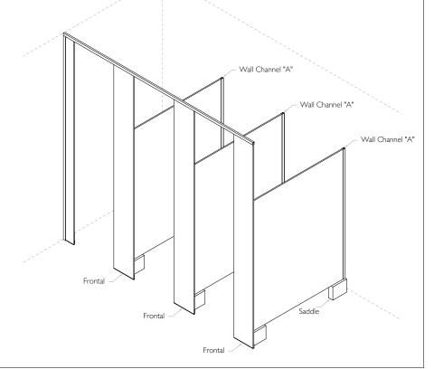
Fit door inserts into the underside of ceiling channel. String line across the fronts to plumb. Once all of the fronts are plumb proceed to screw off the divisions to the back wall and to the back of the frontals.
