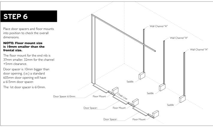
Locate all divisional panels into the rear channels "A" resting onto the saddles.
