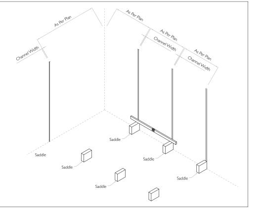
Fix channel "A" to back wall by placing on top of the levelled saddles.
