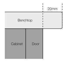
• If cutting a mitre join, cut one benchtop piece first then use this to ensure the corresponding angle on the other benchtop piece is correct, as the walls may not be at 90 degrees - square. This will assist in avoiding open joins.
