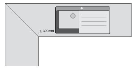
Note: Where possible, joins should always be away from water sources such as sinks to minimise risk of water damage to joins (minimum 300mm).
